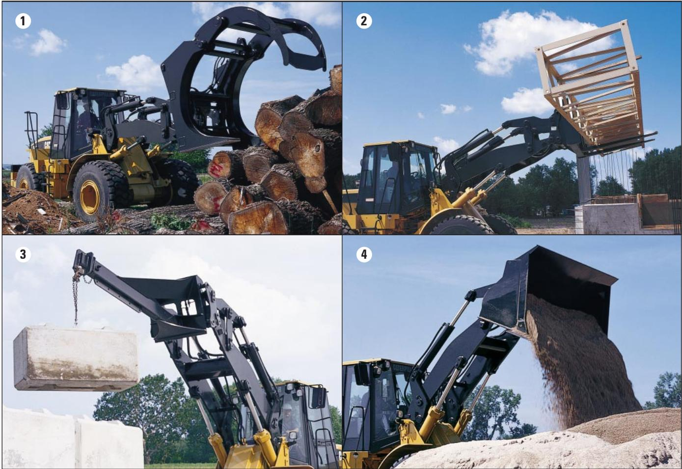
**1 Unloading grapple with kickout.** High volume log loading forks are designed for heavy-duty applications: loading and unloading trucks, sorting, decking, feeding the mill and general millyard work.
