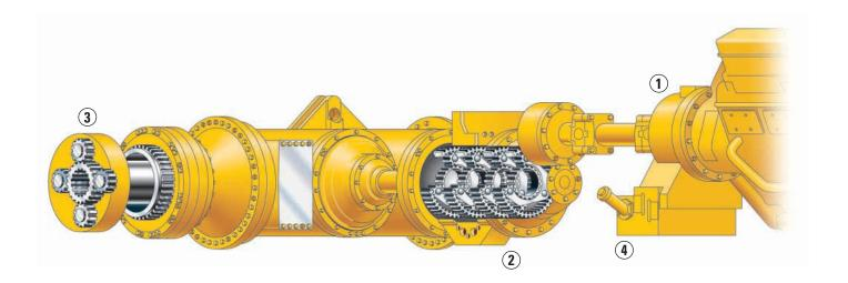
**Transmission.** The Cat seven-speed power shift transmission, matched with the direct injection Cat 3412E Diesel Engine, provides constant power over a wide range of operating speeds.
