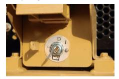
**Ground-Level Battery Disconnect Switch.** Facilitates safe, convenient servicing and maintenance.
