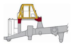
**Box-Section Design.** The 773D frame uses a box-section design, incorporating 21 castings in high-stress areas, with deep-penetrating and continuous wraparound welding. Mild steel is used throughout.
