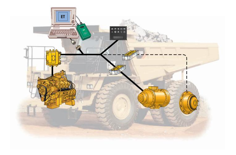
**Integration**. The electronic integration system designed by Caterpillar optimizes overall power train performance, reliability and component life for reduced power train operating cost.
