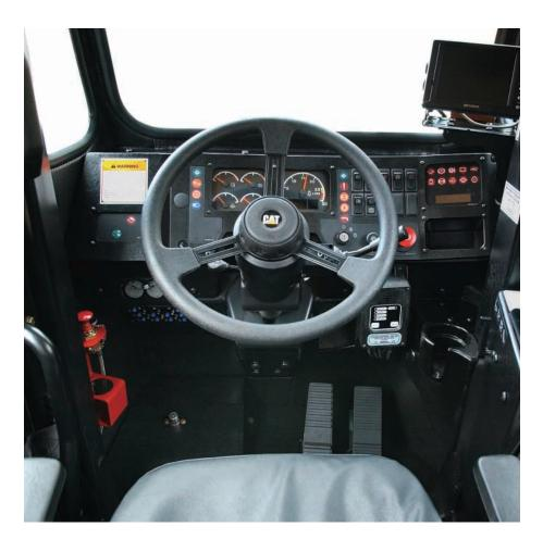
**Ergonomic Layout.** The AD45B operator station is ergonomically designed for total machine control in a comfortable, productive and safe environment. All controls, levers switches and gauges are positioned to maximize productivity and minimize operator fatigue.
