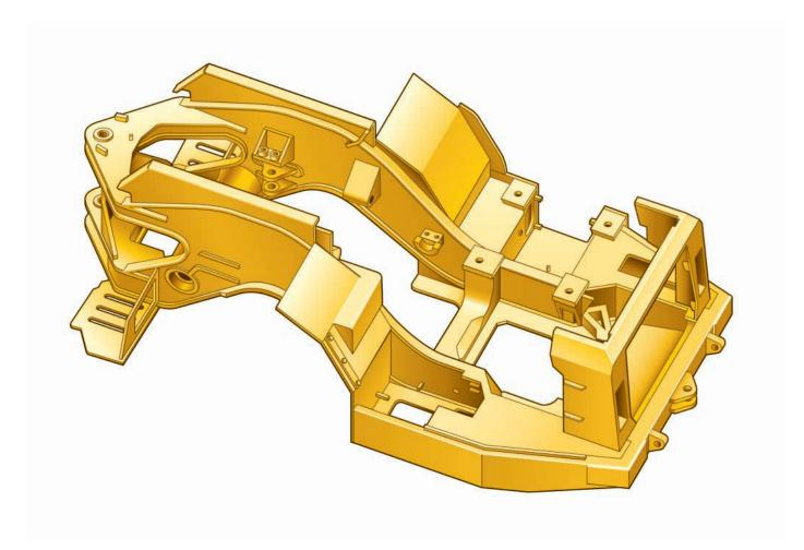
**Frame Design.** The frame incorporates a box-section design with wide and stiff frame beams to handle torque loads. The frame design decreases stress in the hitch area and optimizes suspension geometry. Materials and weld joints are matched to optimize the life of the structure.
