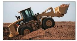
**Ride Control.** The optional Ride Control System improves ride, performance and load retention when traveling over rough terrain. Operators gain confidence moving at higher speeds in load and carry operations decreasing cycle times and increasing productivity.
