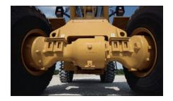
**New! Differential Lock.** Maximize productivity with the new hydraulic locking front differential. This standard feature provides operators with the confidence to maneuver through poor underfoot conditions with 'on the fly' engagement.
