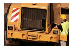
**Counterweight.** The two-piece counterweight is integrated into the 938H design and provides added protection for the lights by incorporating them into the top of the structure.
