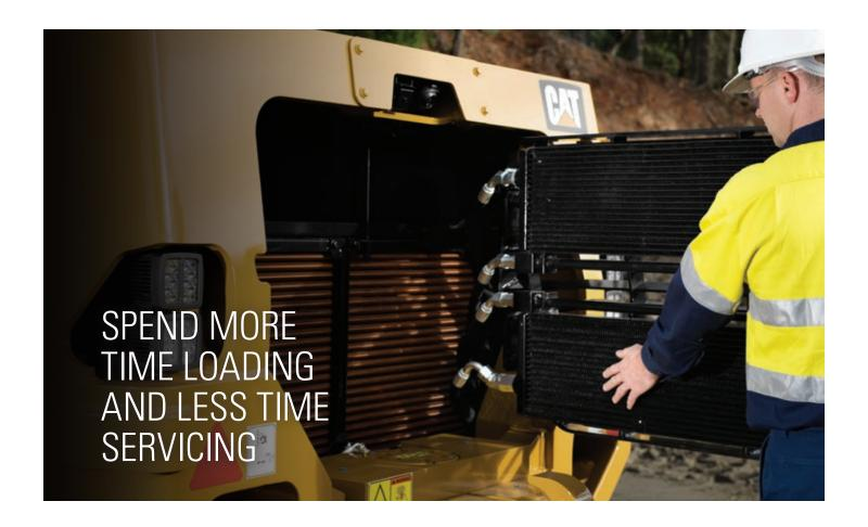
Reduced downtime and maintenance costs are key contributors to the R1700's ability to achieve the lowest possible owning and operating costs. With more robust structures, modular and longer-lasting components, parts commonality, more accessible maintenance areas and extended service intervals, the R1700 can be maintained in less time for less money by fewer people — helping you lower cost per ton and keep your machines hard at work.
