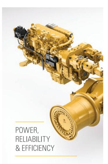
All new levels of power and performance for the R1700 start with the engine — the C13 — which is larger than the previous model. It's a heavy-duty performer with an in-line, 6-cylinder configuration that is turbo-charged and air-to-air aftercooled. In the R1700, this engine is set at a horsepower rating of 257 kW or 345 hp at 2,050 rpm for Stage V engines, and 269 kW or 361 hp at 1,800 rpm for engines that emit equivalent to Tier 3/Stage IIIA or Tier 2/Stage II VR (ventilation reduction).
